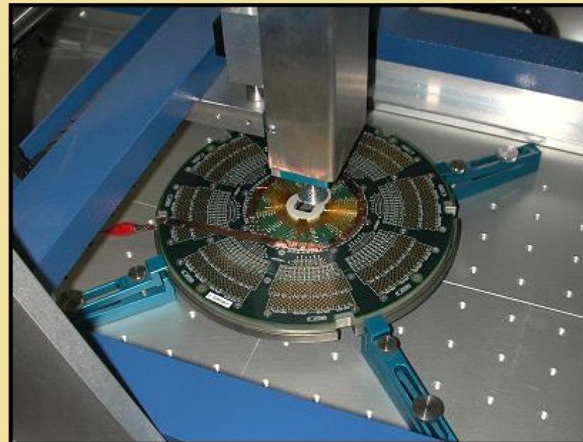
Fine Pitch Probe Card during Machining
