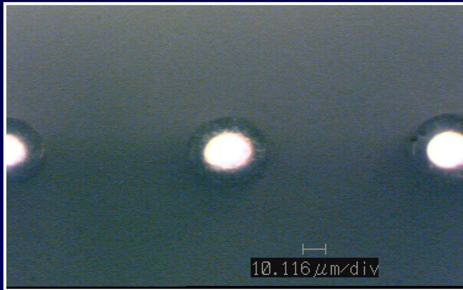
Probes after Non-destructive Cleaning (Mag: 150X)
