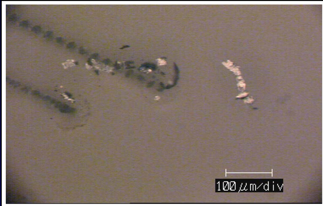
Debris Collection on Cleaning Material Surface and within the Polymer Layer
